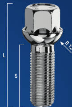
LUG BOLTS M12x1,5 BALL SEAT 17mm HEX (radius 12 mm)
