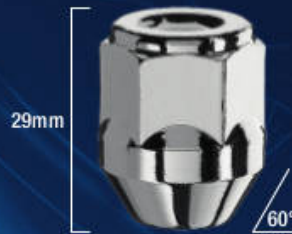
CLOSED LUG NUTS CONE SEAT 21mm HEX
