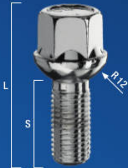
LUG BOLTS M12x1,5 BALL SEAT 17mm HEX (radius 12 mm)
